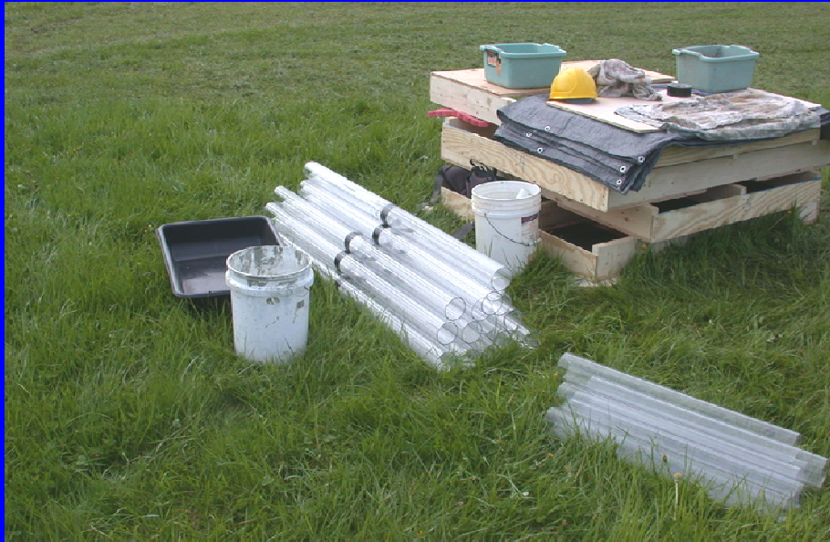
3" core liners (2.5-ft liners taped together with duct tape for each 5-ft core drive).
