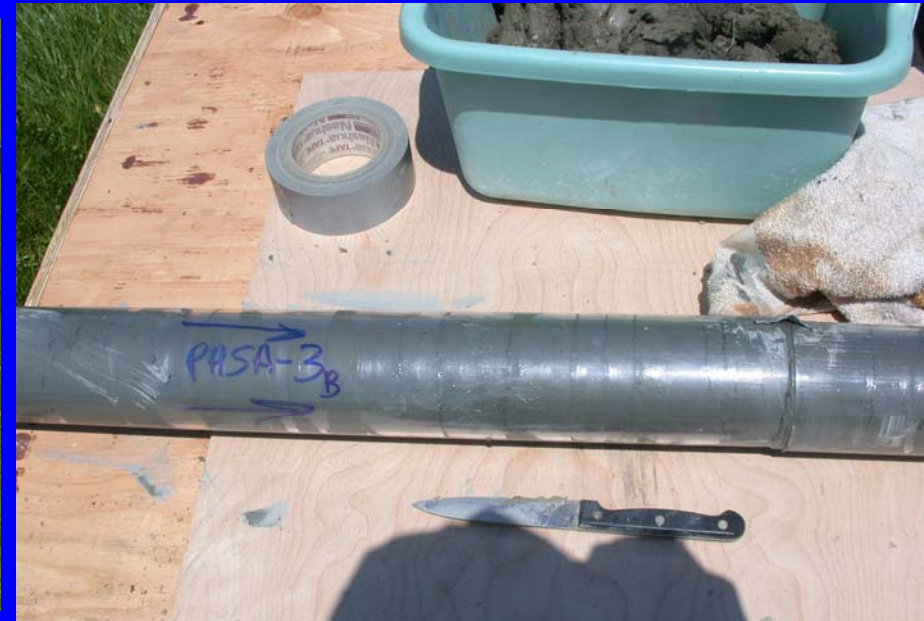
Core sample in liner. 2.5-ft sections are split and taped with duct tape after water is poured out of the liner and space in the liner is filled with waste sediment to prevent the core sample from traveling inside the liner during transport.
