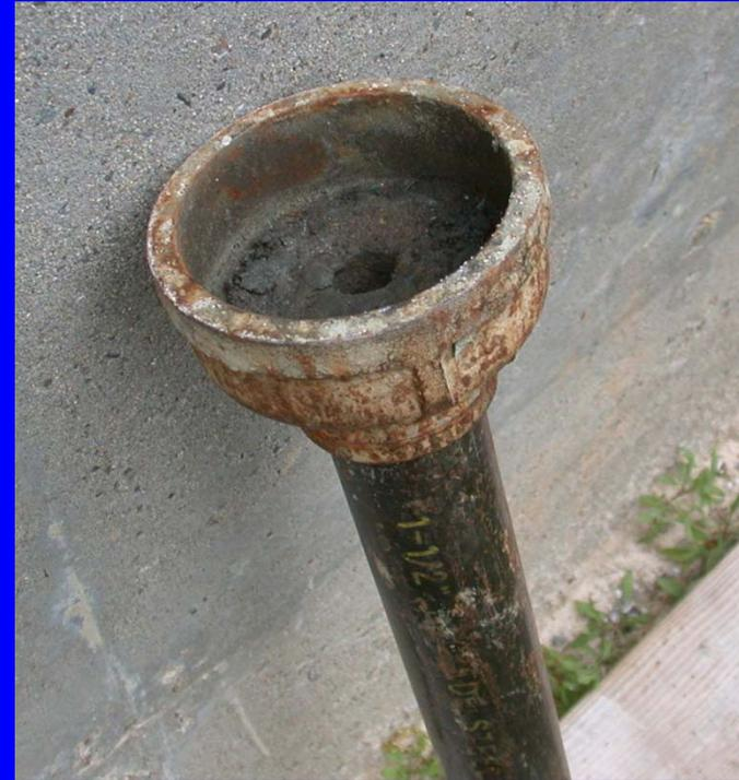
Close up view of bottom of lower half of core driver that fits over 3"ID PVC pipe or 2.5"ID PVC pipe with an end cap. The threads inside this coupling have been removed on a lathe to easily accept the PVC pipe. It should be snug but not tight. A flat platform with a hole to allow air escape has also been mounted with liquid steel epoxy inside the coupling cap as a sturdy, flat, pounding platform for the PVC pipe.
