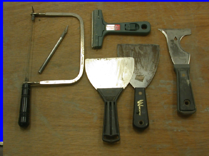
Core splitting, scraping, and shaving tools.
